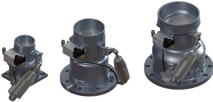
**APPLICATION:** Installed on the compressor inlet to control compressor capacity. During normal operation the valve open and close in response to a control signal to meet the air demand. Stepless or two point capacity controls are available. At the shut-down a check valve stays closed to prevent back flow through the compressor also if the air flow is interrupted. Many solutions are available for stationary or mobile compressors.
