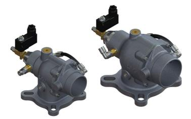
**APPLICATION:** Installed on the compressor inlet to control compressor capacity. During normal operation the valve open and close in response to a control signal to meet the air demand. At the shut-down a check valve stays closed to prevent back flow through the compressor also if the air flow is interrupted.
